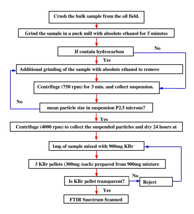
Figure 1. The sample/KBr pellet preparation flow chart.
